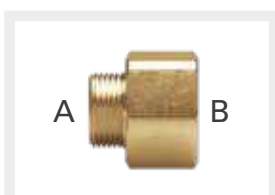
Nipplo ridotti M/F in ottone con filettatura maschio ISO 228 G a battuta piana (A) e filettatura femmina EN 10226 Rp (B) Brass M/F reduced nipples with ISO 228 G male thread with plane end (A) and EN 10226 Rp female thread (B)
